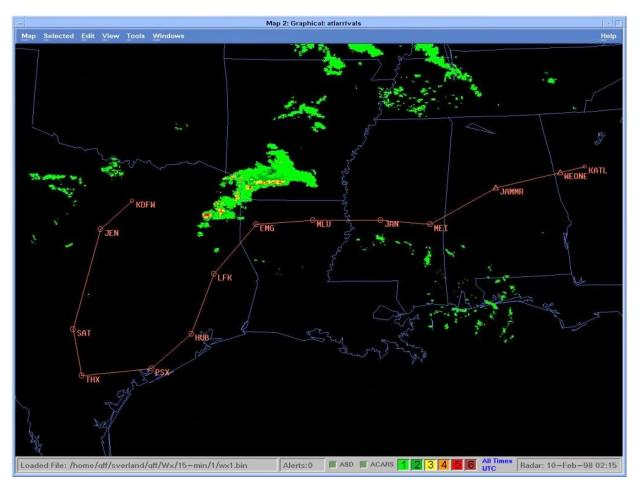
This screen capture showing an airline aircraft situation display screen capture from 1999 displays an extensive ATC retour around a small area of developing thunderstorms east of DFW airport.
